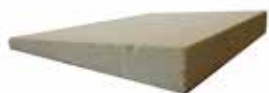
The KÖSTER Hydrosilicate Taperd Board is a specially designed board that prevents thermal bridges between the external and the internal walls or the ceiling. It is delivered in the size 500 x 380 x 60 to 20 mm.
